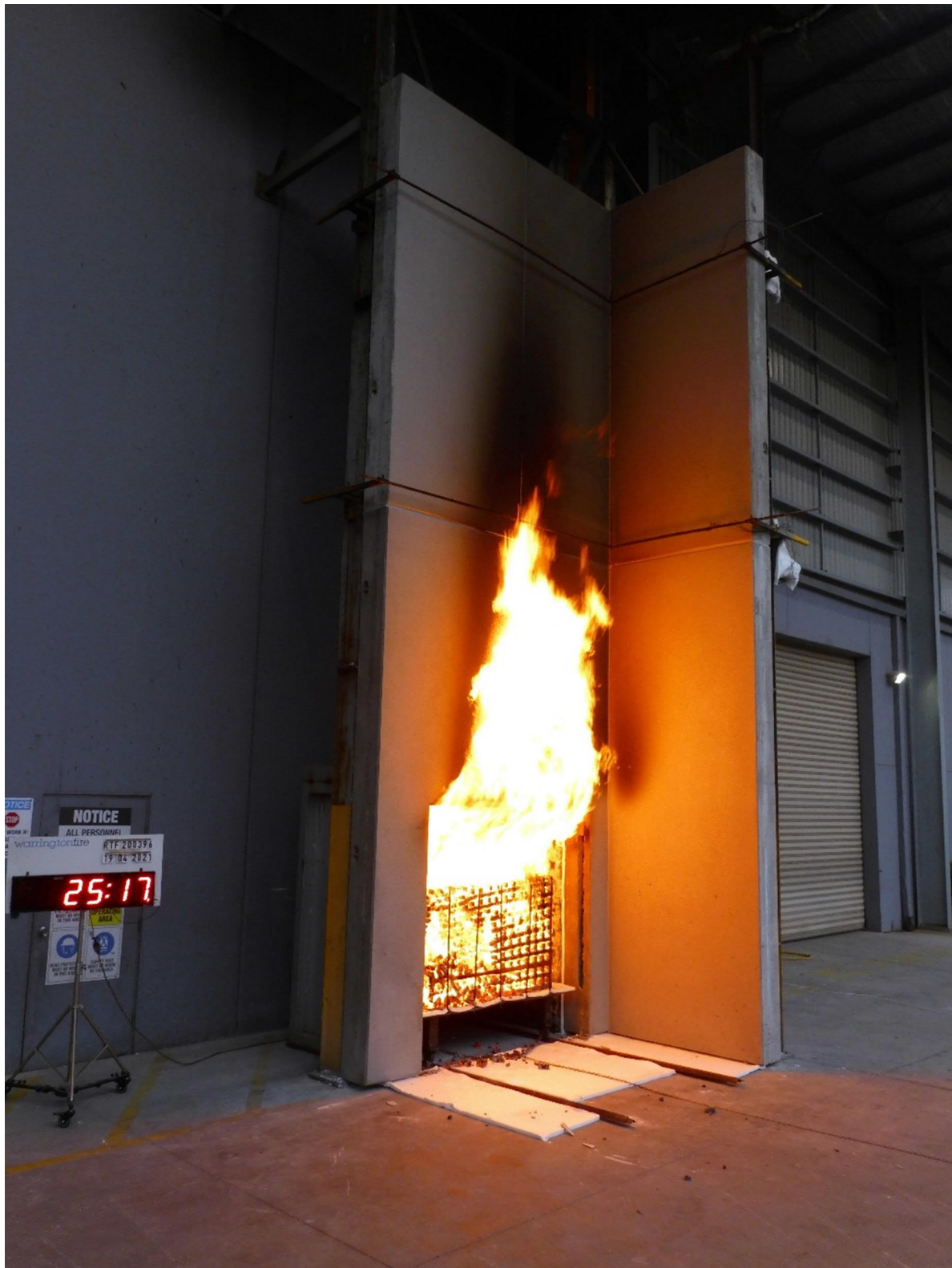
Figure 31 The external wall system during the test – 25 minutes 17 seconds after crib ignition
