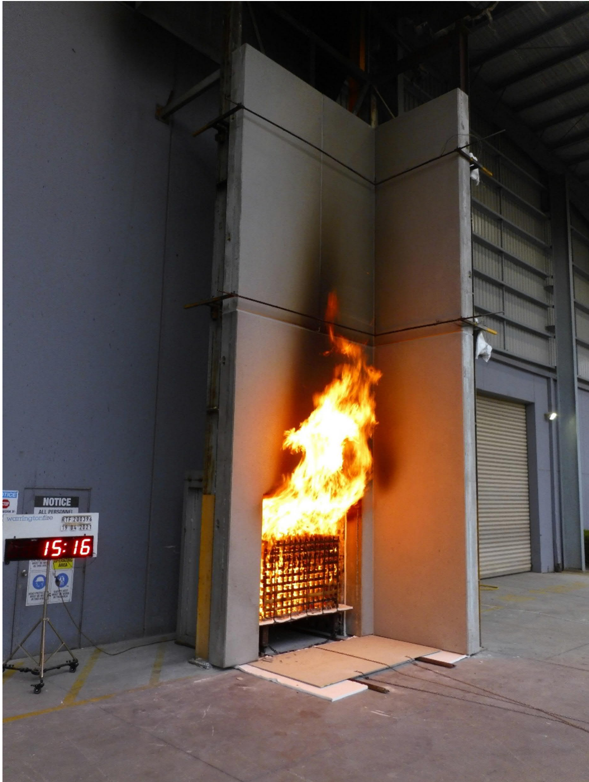
Figure 29 The external wall system during the test – 15 minutes 16 seconds after crib ignition
