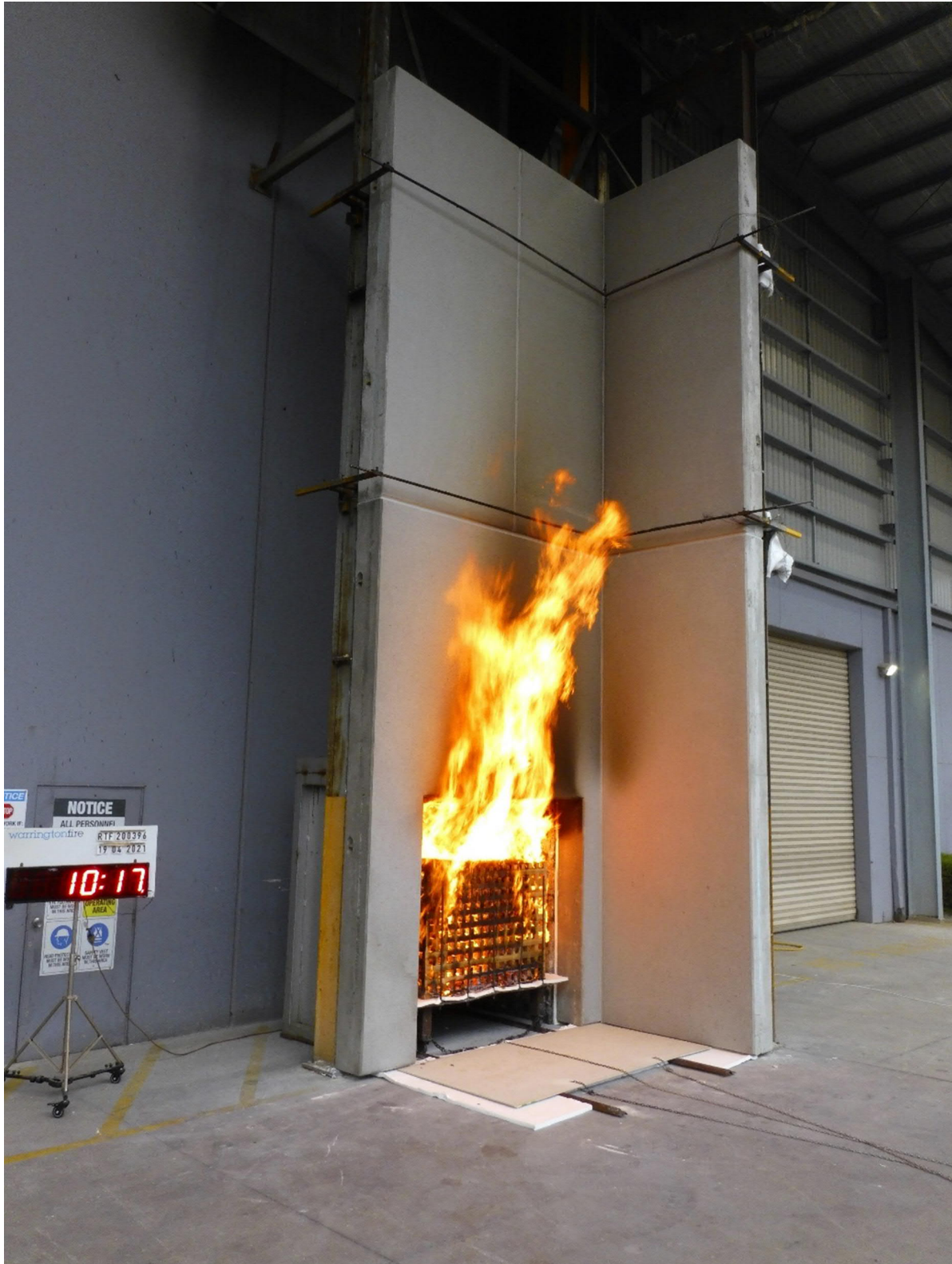
Figure 28 The external wall system during the test – 10 minutes 17 seconds after crib ignition
