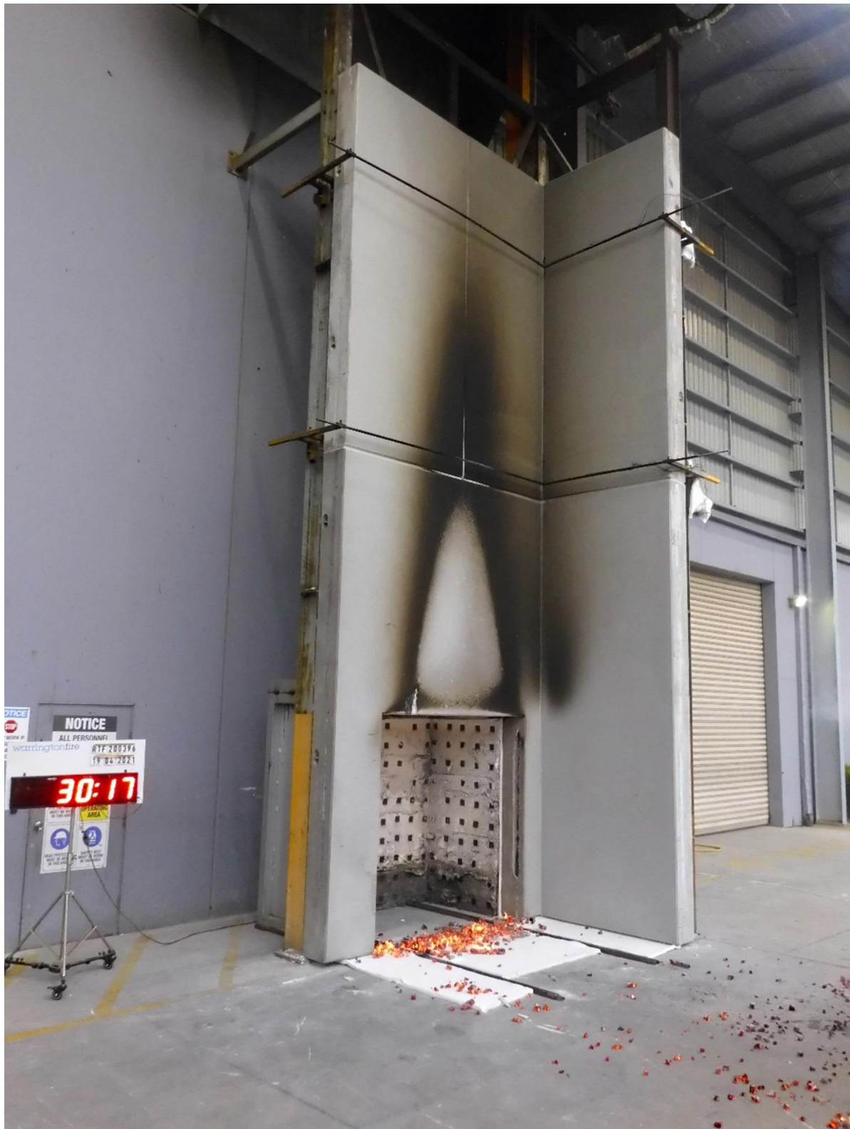
Figure 32 The external wall system during the test –during removal of the crib, 30 minutes after ignition of crib 12
