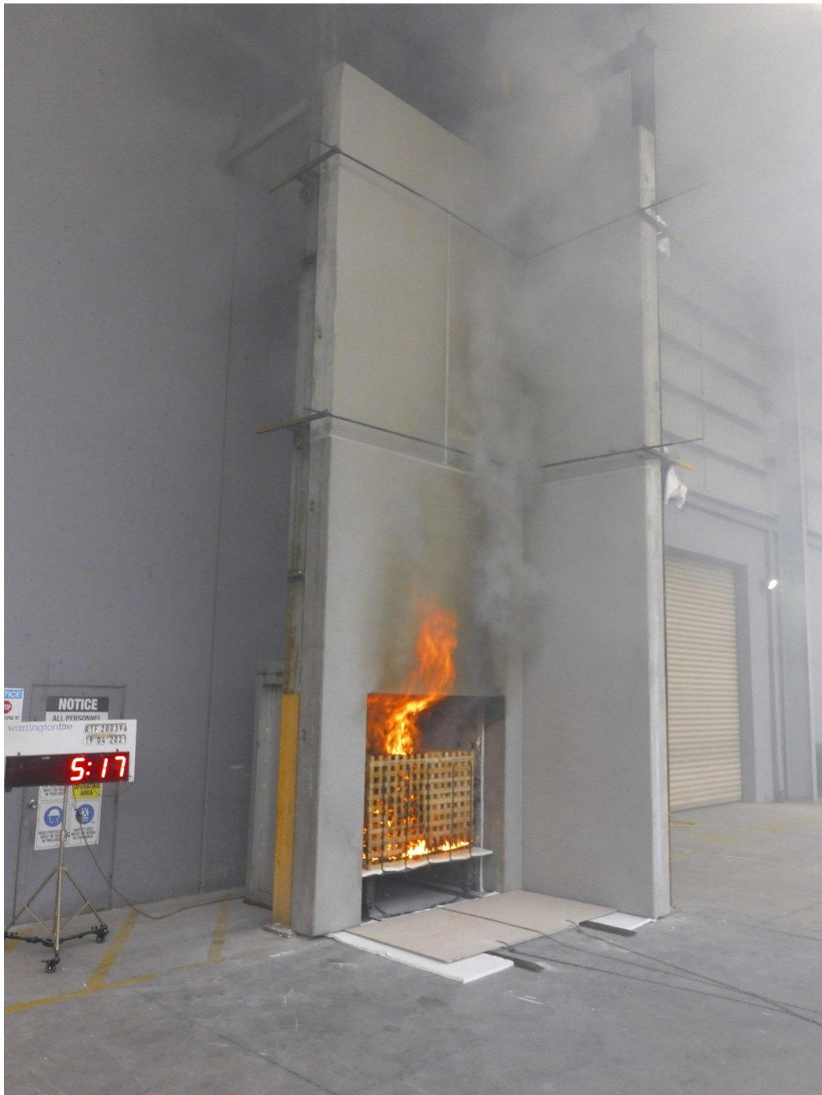
Figure 27 The external wall system during the test – 5 minutes 17 seconds after crib ignition
