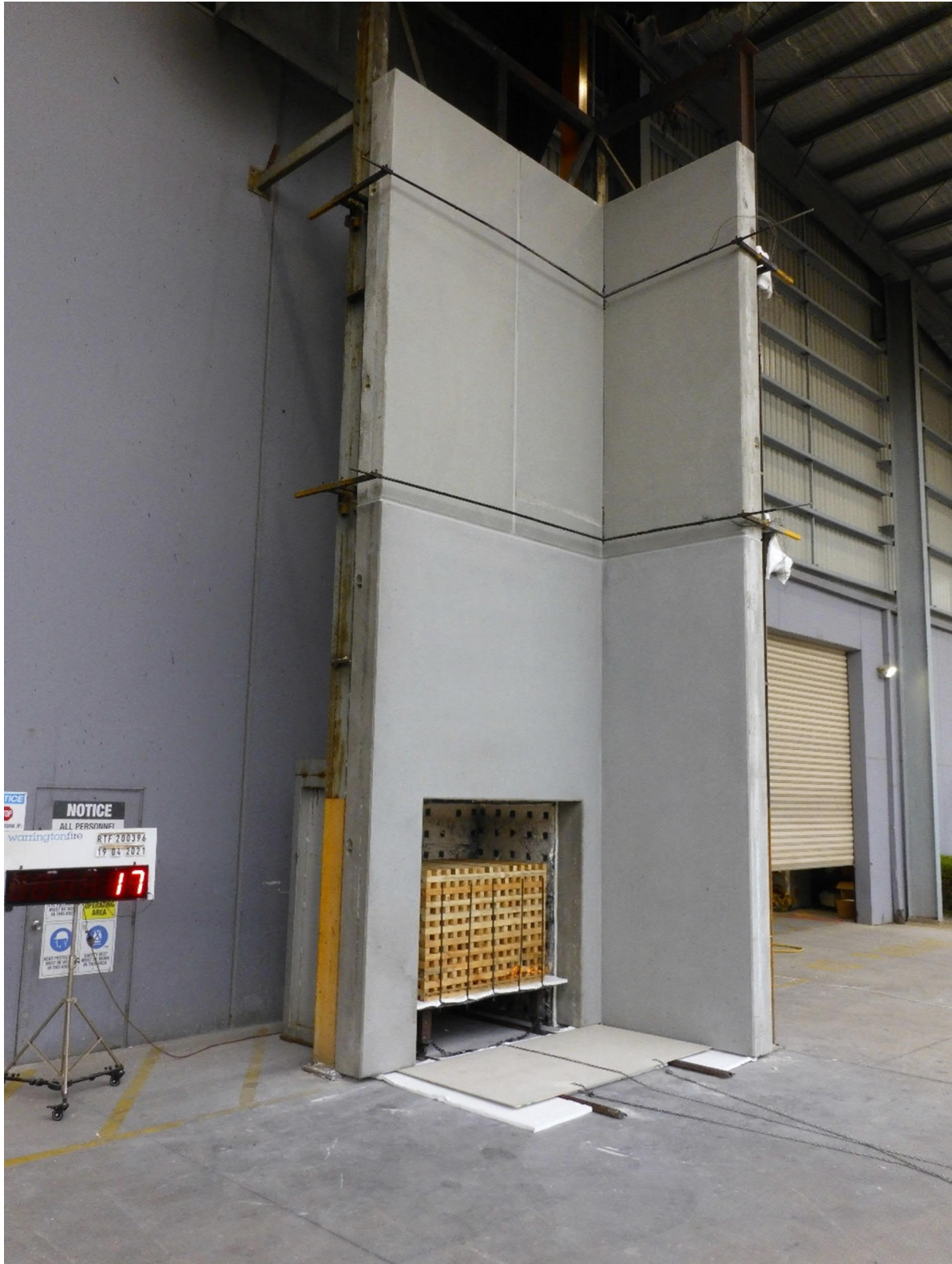
Figure 26 The external wall system during the test – 17 seconds after crib ignition
