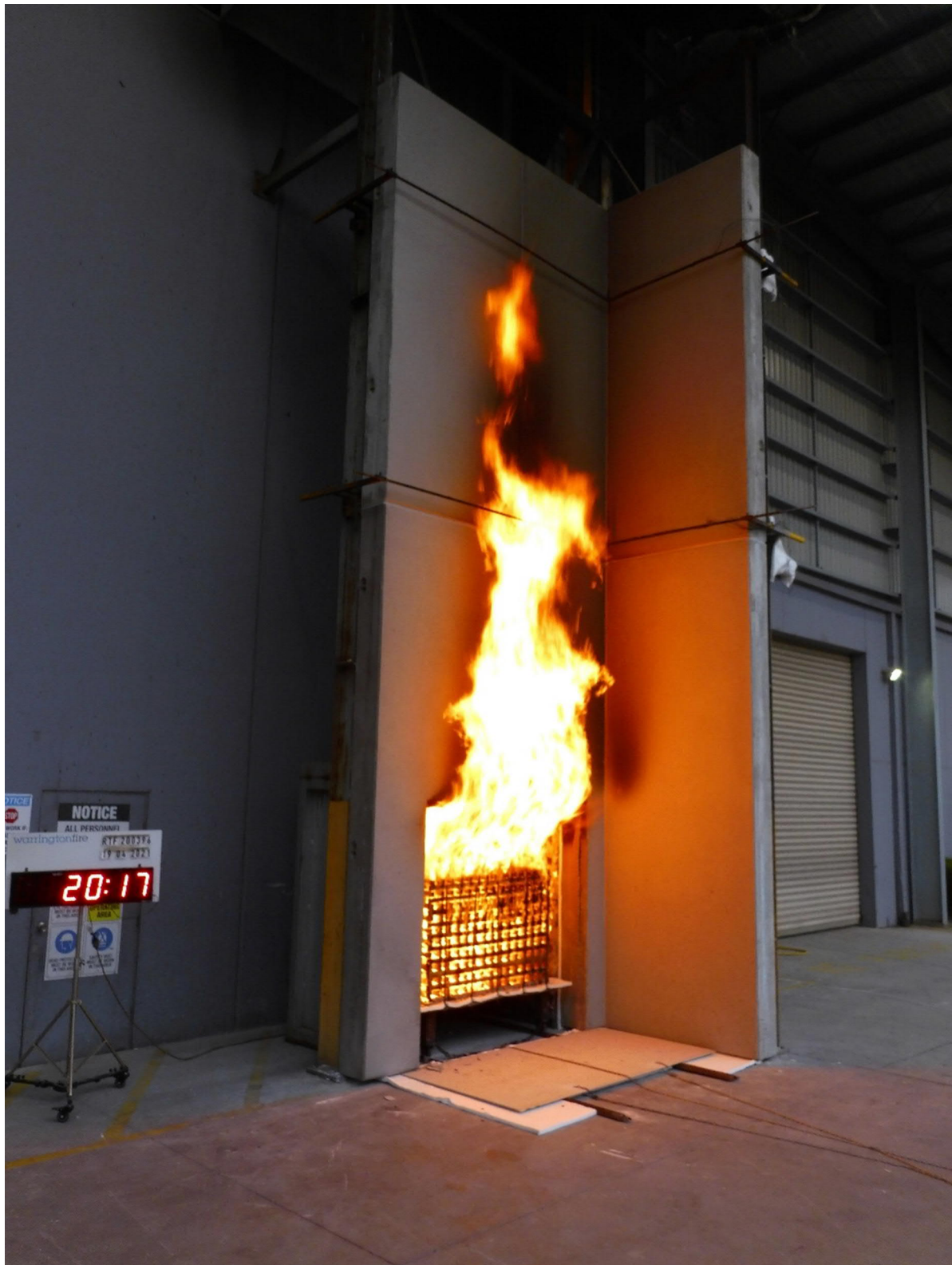
Figure 30 The external wall system during the test – 20 minutes 17 seconds after crib ignition
