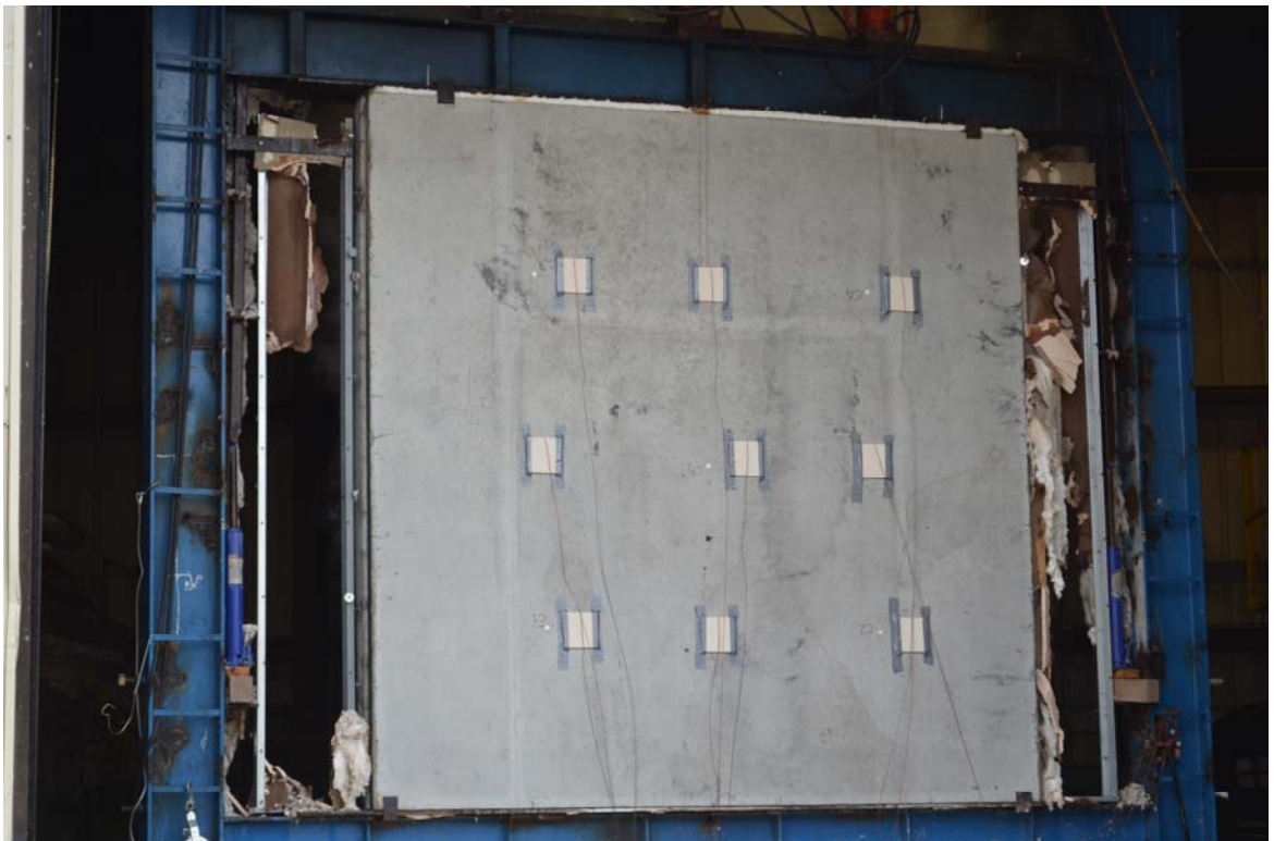
Figure B-12. Unexposed Face following the Hose Stream Test.
