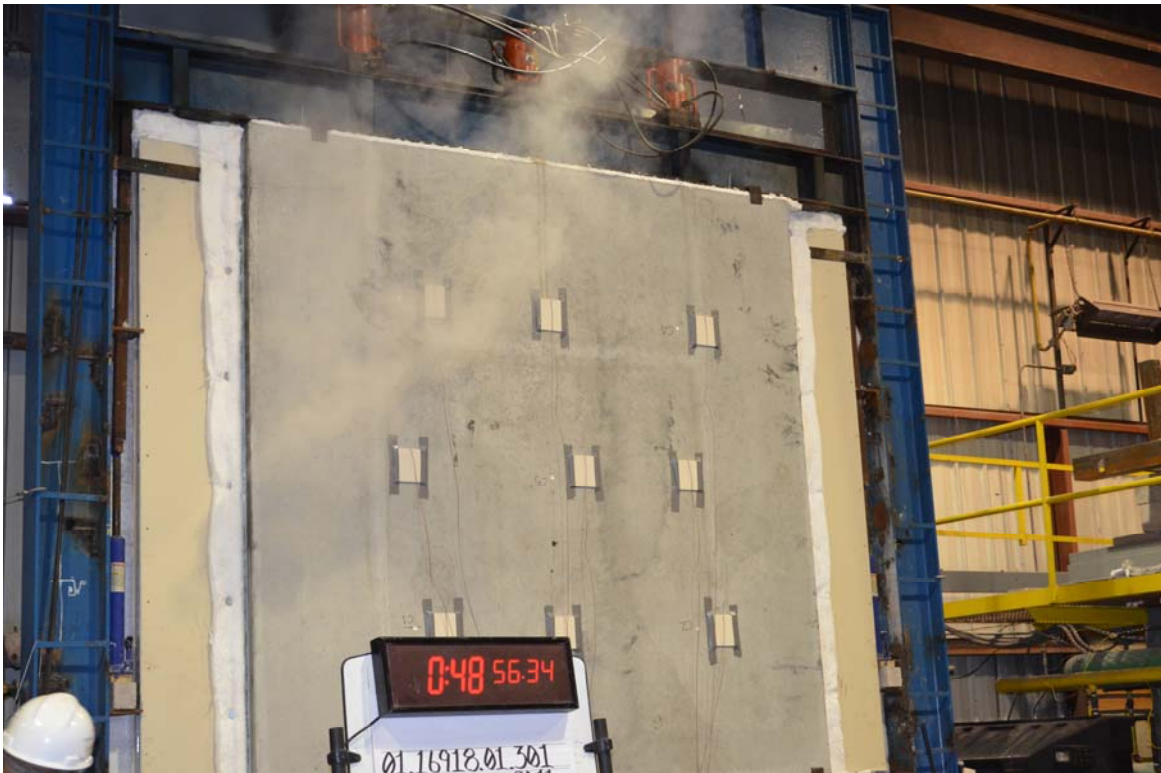
Figure B-6. View of Wall Showing Steam Escaping from Left Side at 48 min.
