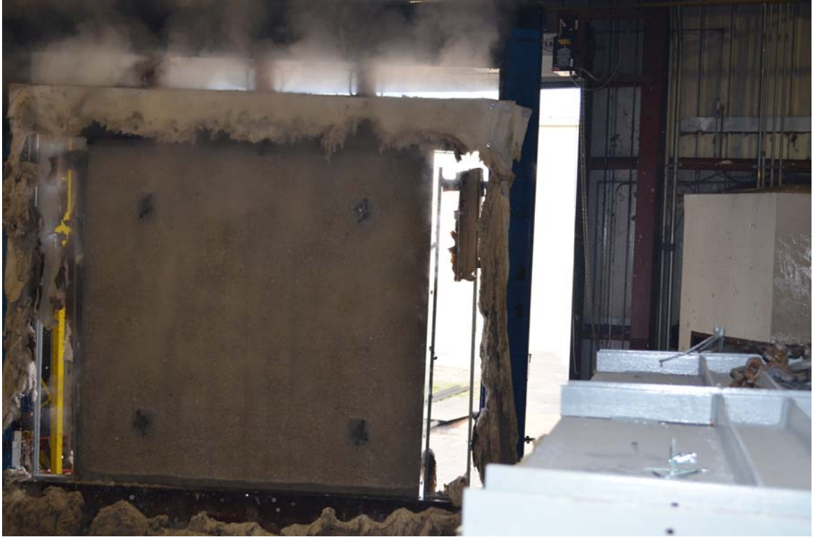
Figure B-11. Exposed Face following the Hose Stream Test.
