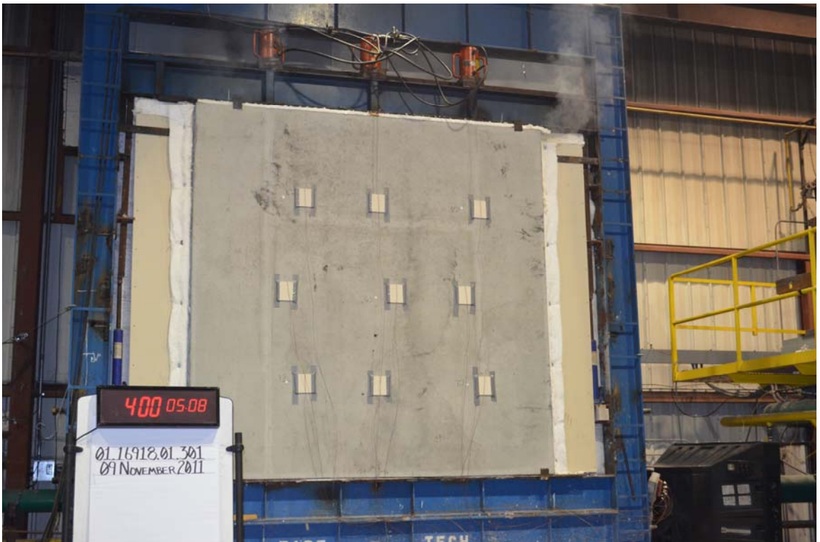
Figure B-8. Unexposed Wall at End of 4-hr Fire Test.
