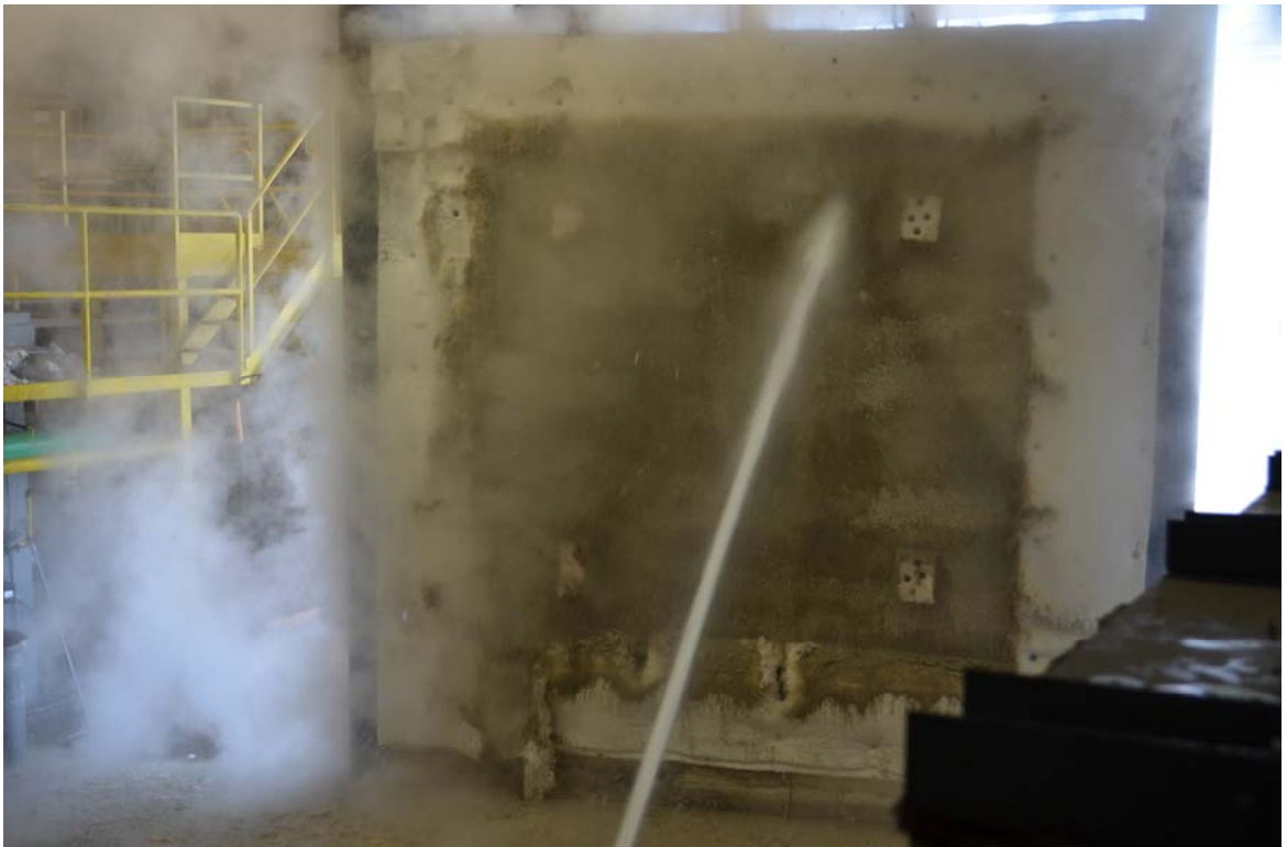
Figure B-10. Hose Stream Test
