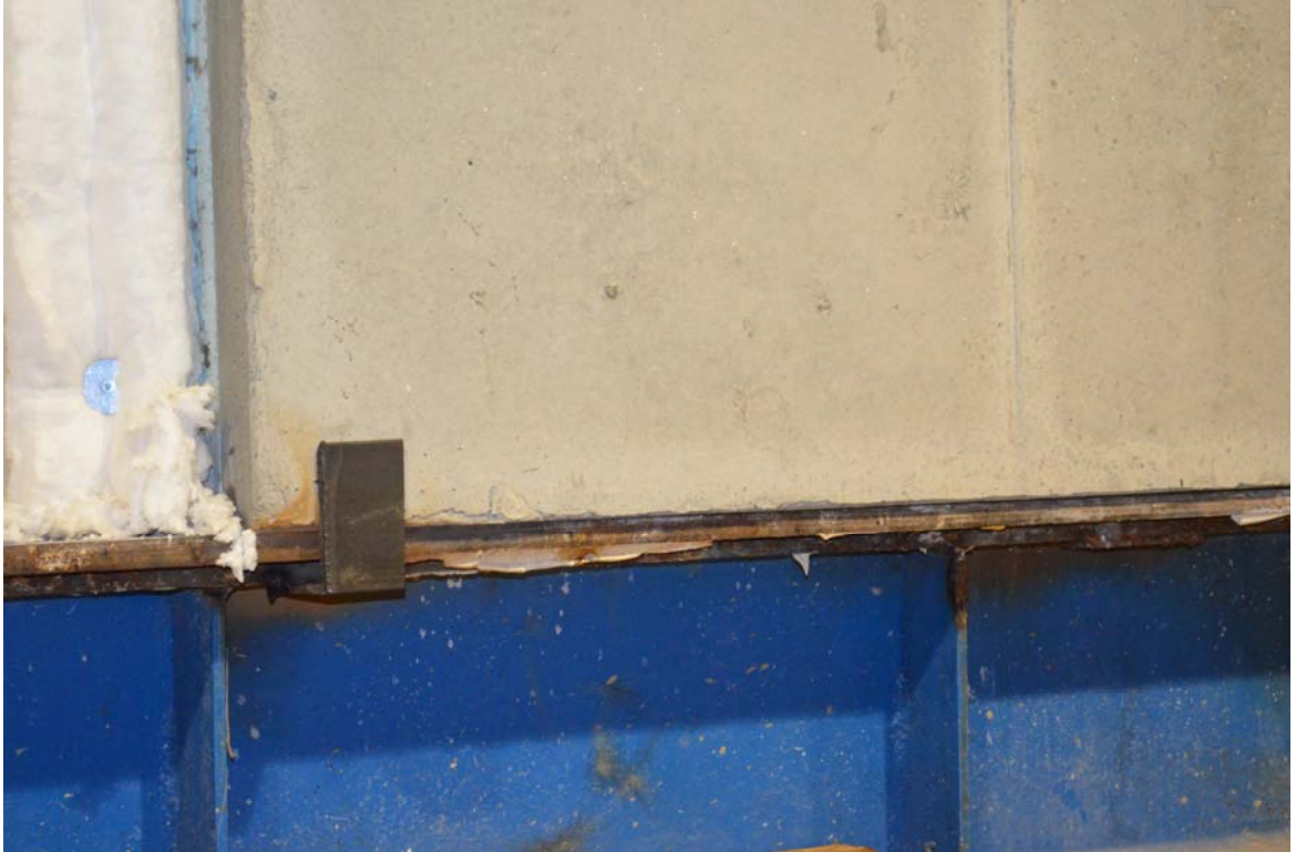
Figure B-7. Close-Up Showing the Unexposed Wall Resting on the Test Frame at 136 min.
